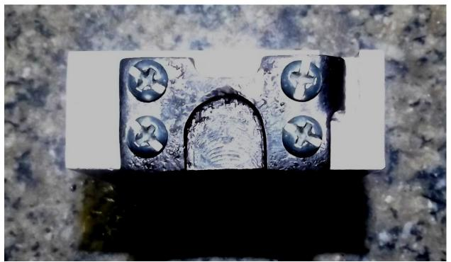
In the photograph above, the selector stop is fastened to the fixture with the screws. In the photograph immediately below, a diameter 0.500" endmill is centered to the depression, touched off, lowered to the correct depth and the cut is usually made in a single pass. Note that the specification of the width of the depression is 12,6mm and the diameter 0.500" endmill will give a slight width increase to 12,7mm. This does not affect function.
