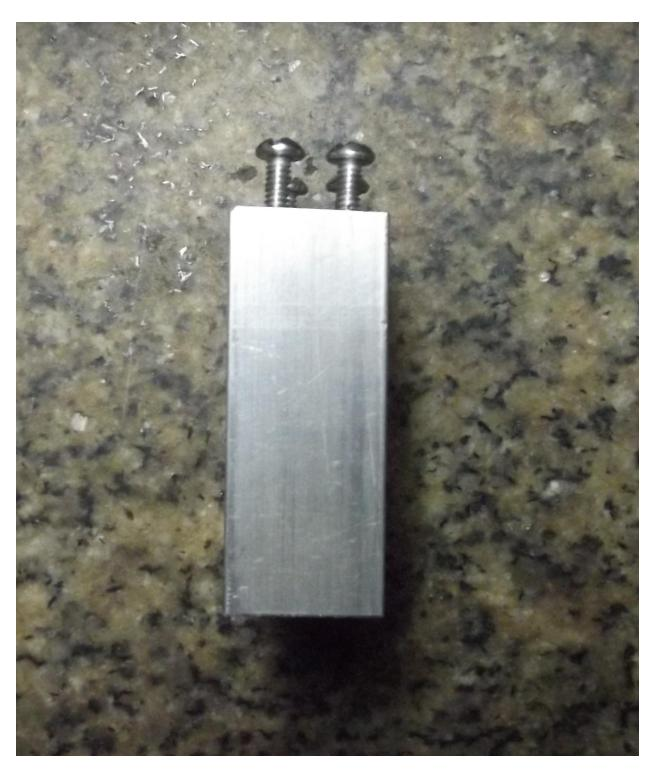
In the photograph above, you can see a simple tool that allows holding the selector stop while the depression depth is increased. It is made from aluminium with a pattern of tapped Nr. 6-32 UNC holes. The top of this fixture has an angle of 2-degrees 30-minutes to closely match the 2-degree 33-minute theoretical angle of the lower plane of the stamped or milled frame.
