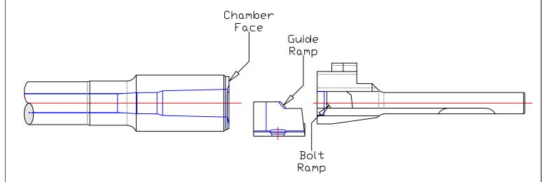
Insert 2,5mm Thick Gauge Between Bolt Face And Chamber Face.
