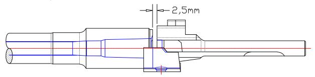
Insert 2,0mm Thick Gauge Between Bolt Face And Chamber Face.
